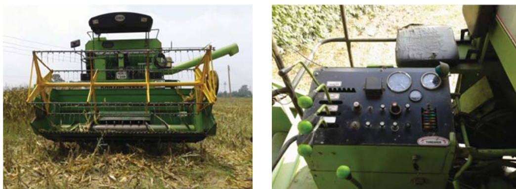
Figure 3. View of developed cutter bar header and control unit of combine harvester
