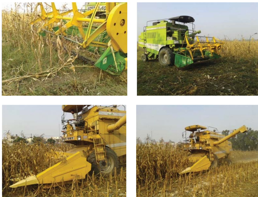
Figure 12. Another view of cutter bar and snap roll maize header during field operation
