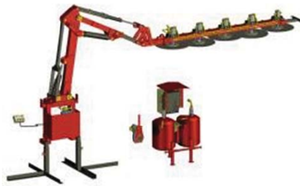
Figure 6. A Schematic view of various components of pre-pruner
