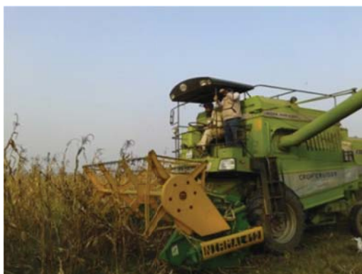
Figure 10. A view of lodged maize harvesting with combine equipped with cutter bar type maize header
