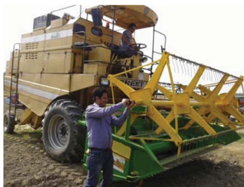
Figure 9. Measurement of reel rpm with tachometer at various engine speeds
