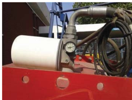
Figure 8. Pressure gauge for checking hydraulic oil pressure
