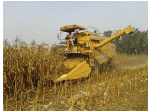
Figure 5. A view of maize harvesting with combine equipped with snap roll maize header
