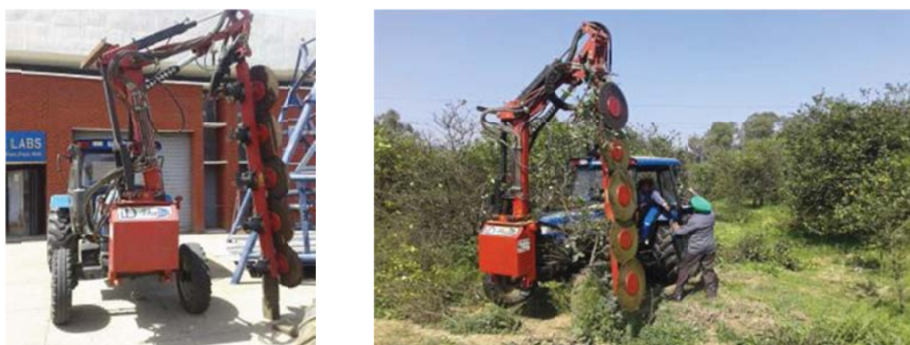
Figure 7. A view of tractor operated pre-pruner lab and field experiment
