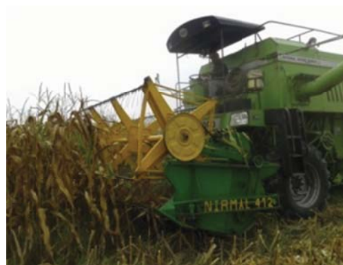
Figure 11. A view of dislodged maize harvesting with combine equipped with cutter bar type maize header
